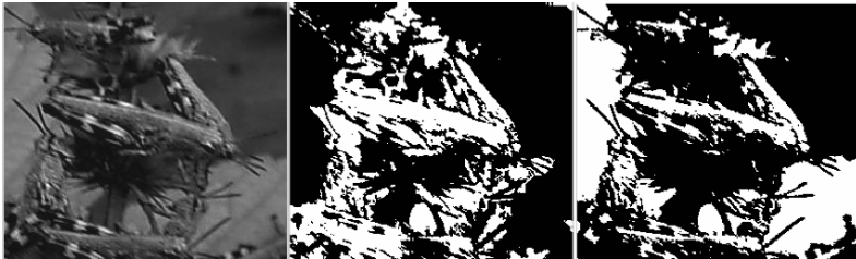
Fig. 2. Locusts from a short distance (left, converted as a gray-scale image) and the segmentation results (middle: result of open operation; right: result of PCNN at n=2 )
